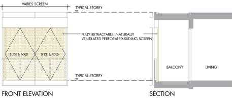
\* The screen design is provided for aesthetic uniformity of the development. Materials to be of aluminium with fluorocarbon finish. Panel design may vary for different unit types. Total free opening for perforated screen shall not be less than 50% of the panel. Drawing not to scale, and none can be regarded as representation of fact. The Purchaser is required to refer to the Management for any additional details.
